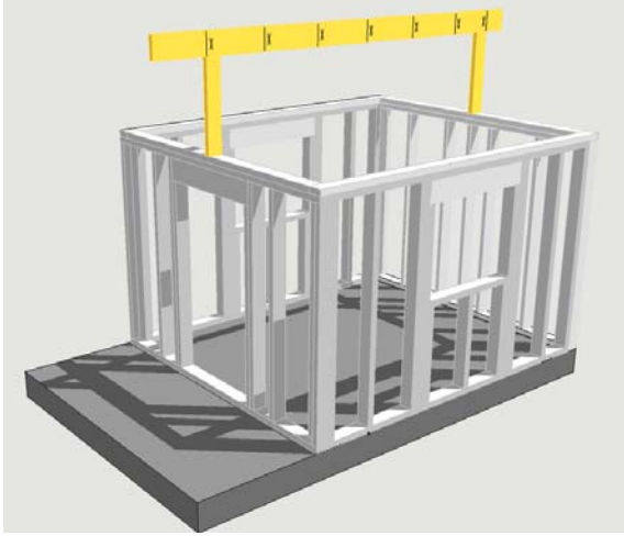
Ridge board & Gable stud 설치
