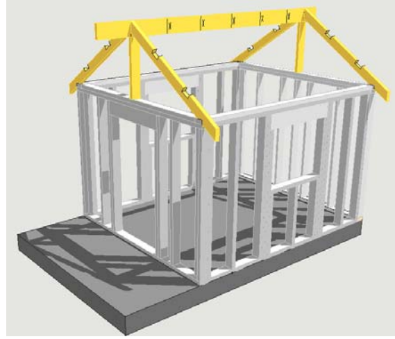
Lookout rafter 설치
